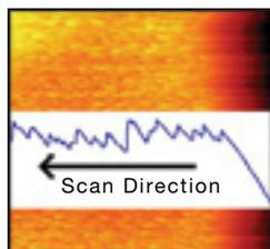
**Figure 4:** Lateral force image and line trace at 128 K.
