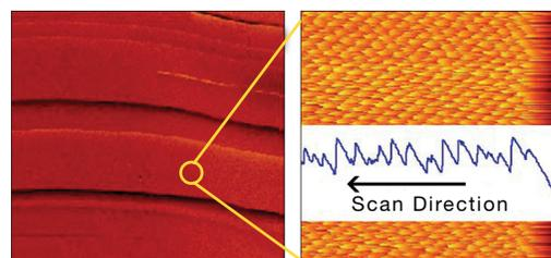
**Figure 2:**  $2 \times 2 \mu\text{m}^2$  deflection (left) and  $10 \times 10 \text{ nm}^2$  friction trace (right) showing stick-slip behavior with periodicity equal to the lattice constant of NaCl ( $5.65 \text{ \AA}$ ); raw data is shown without filtering.
