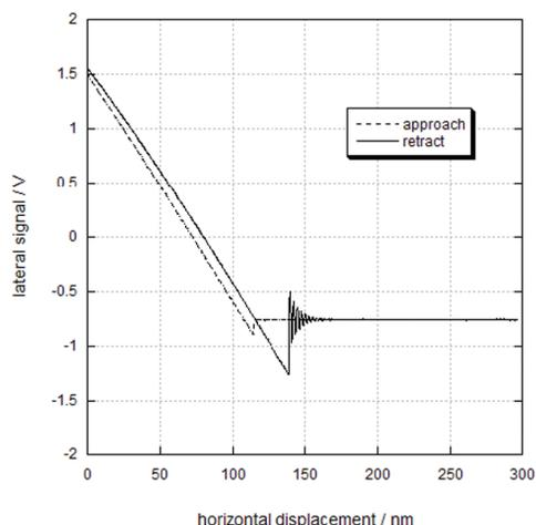
**Figure 8:** Lateral force-distance curve for a colloidal probe against a vertically-oriented (110) plane of a GaAs crystal.
