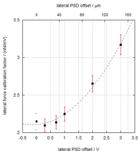
**Figure 9:** The lateral force calibration factor versus lateral PSD offset in volts (out of ~6V) and microns (where the width of each PSD sector is 1.3 mm). Dashed line is a parabolic curve fit. The absolute uncertainty is a percentage of the calibration value and, therefore, increases with increasing displacement of the laser spot relative to the center of the PSD.
