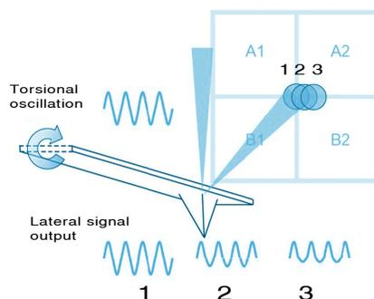
**Figure 7:** Schematic representation of the cantilever undergoing a torsional, sinusoidal oscillation at different lateral offsets of the laser spot relative to the PSD. The lateral signal ( $A1+B1-A2-B2$ ) output from the PSD depends on laser spot position. If it is offset from the center of the PSD, the output signal will be distorted from the sinusoidal signal that represents the true mechanical behavior.
